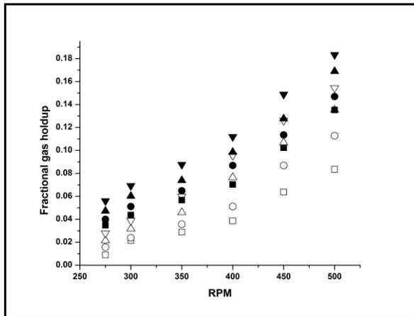
**Figure 9 - Relation between fractional gas holdup with rotational speed at various immersion depths of 20cm (□)sparging and(■)induction, 25cm (○)sparging and (●)induction, 30cm (△)sparging and (▲)induction, 35cm (▽)sparging and (▼)induction.**
