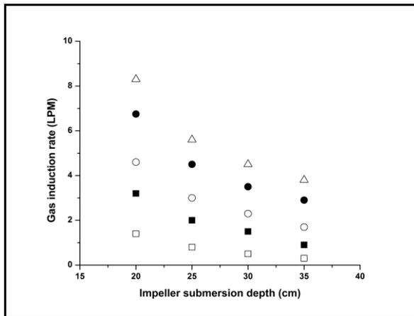
**Figure 6 - Relation of gas induction rate with impeller submersion depths at (□)300 rpm, (■)350 rpm, (○)400 rpm, (●)450 rpm, (▼)500 rpm**
