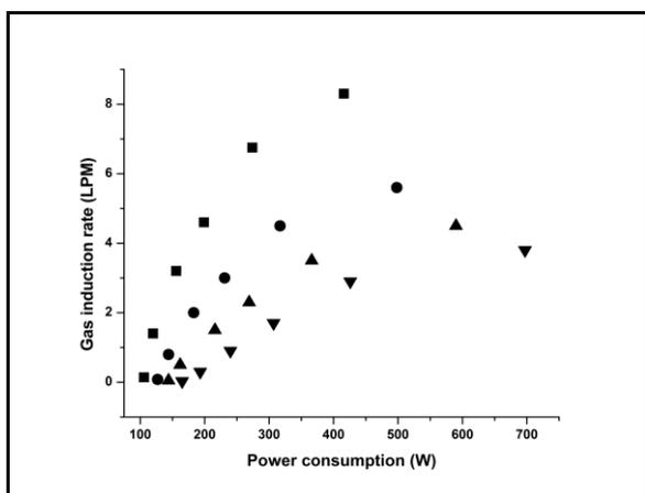
Figure 5- Relation of gas induction rate and power consumption at impeller immersion depths of (■)20cm, (●)25cm, (▲) 30cm and (▼)35cm
