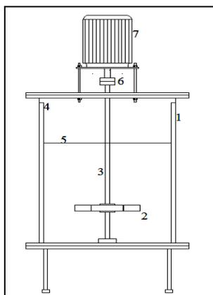
**Figure:1 Gas inducing mechanically agitated contactor**
