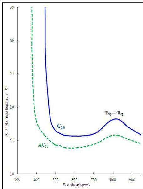
**Fig. 1 Optical absorption spectra of  $\text{Li}_2\text{O}-\text{ZrO}_2-\text{SiO}_2$  glasses doped with 0.20 mol % of CuO recorded at room temperature before and after crystallization**
