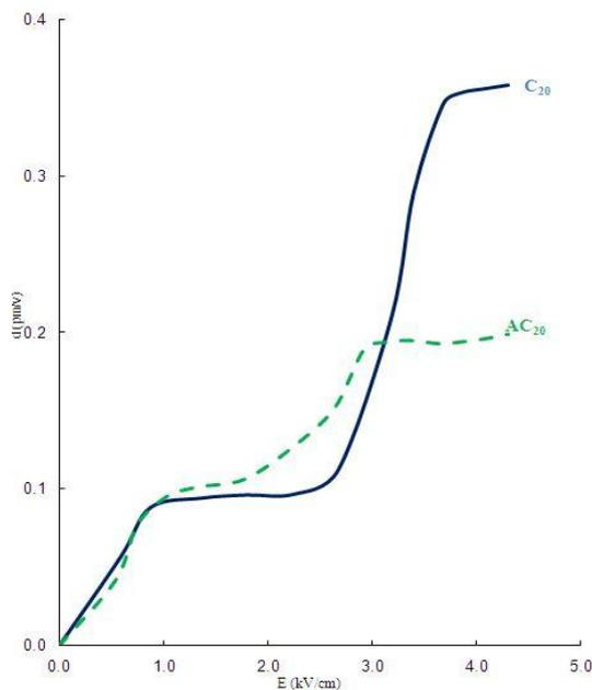
**Fig. 3 Dc-field dependence of the effective second order susceptibility for the Li<sub>2</sub>O–ZrO<sub>2</sub>–SiO<sub>2</sub> glasses doped with 0.20 mol % of CuO before and after crystallization**
