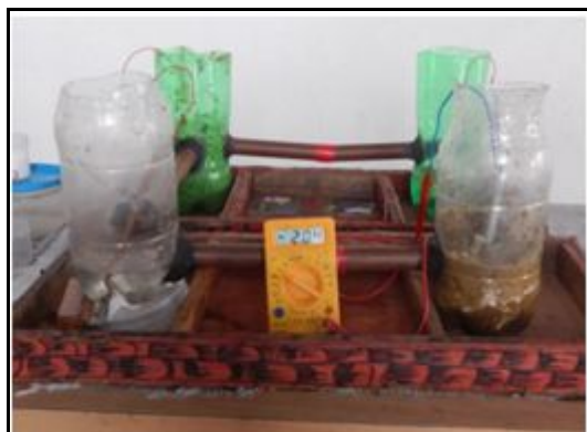
Fig. 2 Microbial fuel cell with two cathodes and one anode
