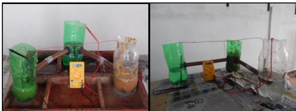
Fig. 1 Microbial fuel cell with two anodes and one cathode
