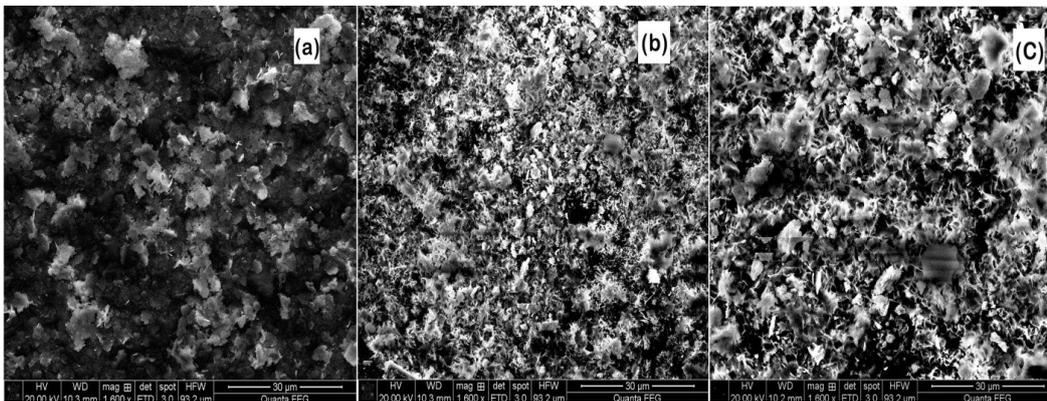
**Fig 2 (a-c): SEM micrograph of CdO thin films (a) 10 dip (b) 15 dip (c) 20 dip****Elemental Analysis:**
