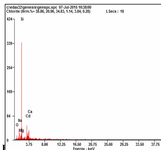
Elemental analysis of CdO thin films was carried out by EDX. Fig. 3 represents the EDX spectrum of CdO thin film. EDX analysis confirms the presence of Cd and O elements in the prepared CdO film.
