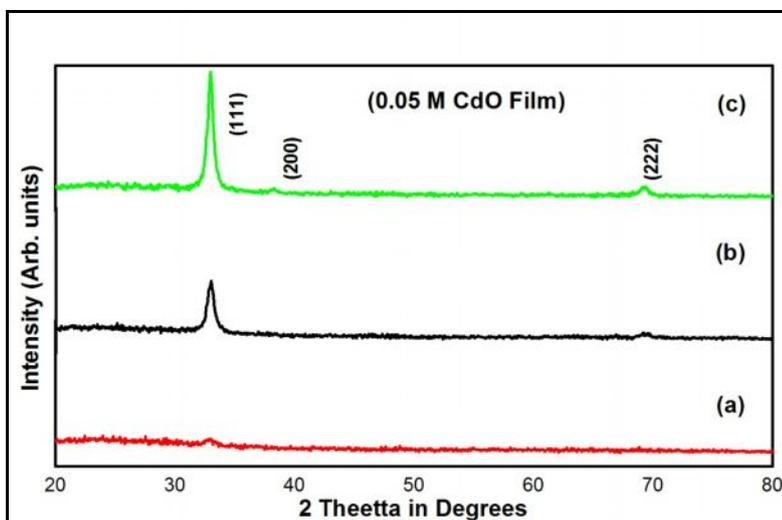
Fig. 1: CdO thin films of 0.05 M at (a) 10 dip (b) 15 dip (c) 20 dip
