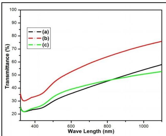
Fig 4: Transmission spectra for CdO thin films (a) 10 dip (b) 15 dip (c) 20 dip
