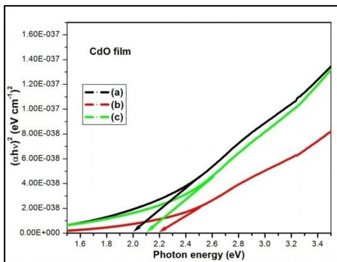
**Fig 5: Optical Band Gap CdO thin films (a) 10 dip (b) 15 dip (c) 20 dip**
